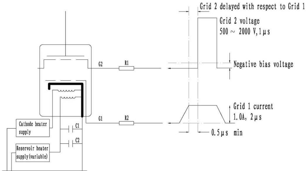
R1, Grid 1 series resistor, 12 W vitreous enameled wire wound is recommended, its impedance matches with the trigger's circuit impedance.
